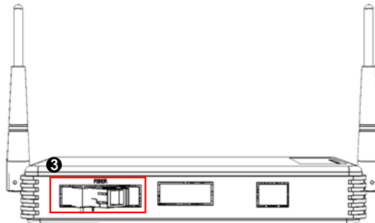
Figure 4. Rear Panel for 4 ports 10/100/1000Mbps RJ-45; built-in IEEE802.11n WiFi and 1 port 100/1000Mbps fiber optics uplink Residential Gateway
